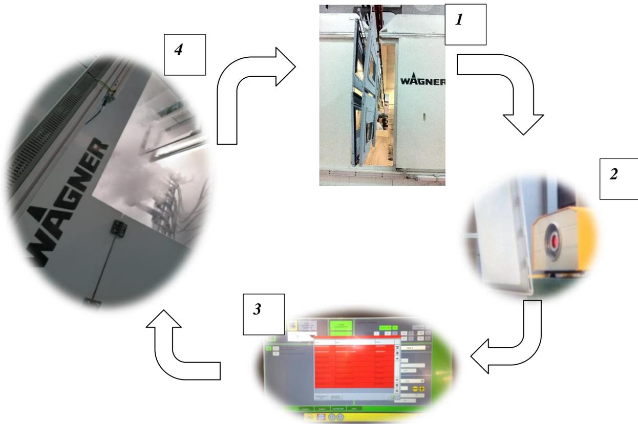
The data received is sent instantly to a PC and, thanks to the software that has been developed, various actions can be taken: from reporting an anomaly to stopping the enamelling line with an alarm
