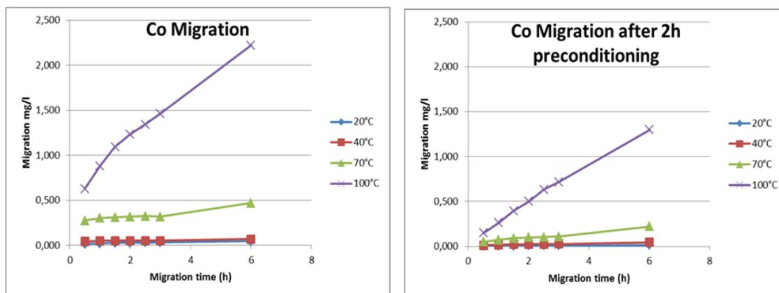
Figure 6 : Migration of Co out of direct on enamel formulation A
