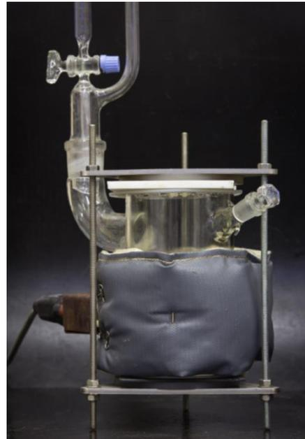
*Figure 1: used test equipment to test the migration at 20°C-40°C-70°C (6 migration tests together) and to test the migration into boiling food simulant (test equipment of EN ISO28706-2).*
